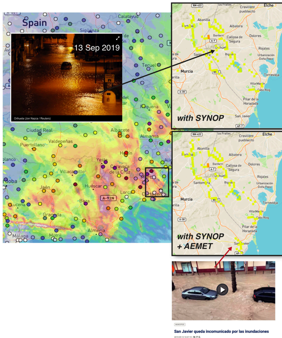
Figure 16: Gauge-adjustment can be by combining SYNOP and existing dense gauge network; e.g. with AEMET over Spain.
