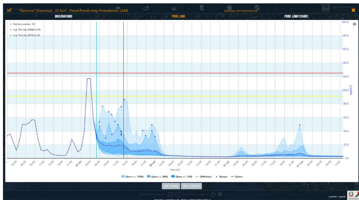
Figure 7. Discharge predicted, in ensemble probabilistic mode, by the Italian Civil Protection river discharge model for the Varenna catchment in the central part of Liguria.
