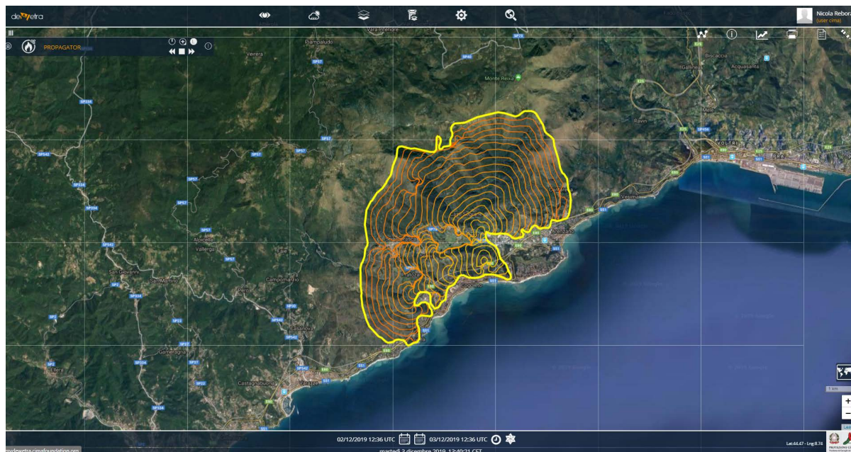
Figure 18. Real-time simulation of Propagator initialized with the ignition area that has been reported at the beginning of the Cogoletto fire event by Liguria Regional firefighters and with the wind conditions observed through the weather stations available in A4Lig.
